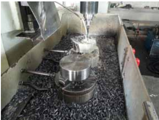
Scenes of Production (Anchor Head Drilling)
