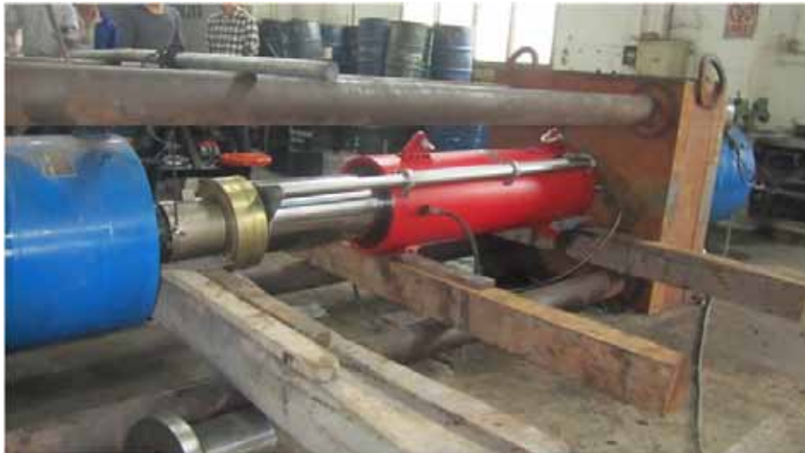
TMG Lifting Jack under Load Test
