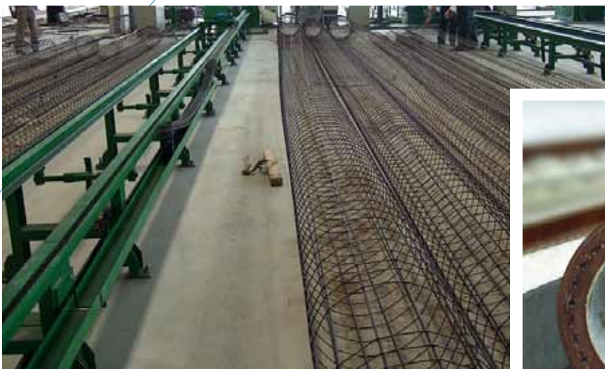
PC Bar used in Concrete Spun Piles Production
