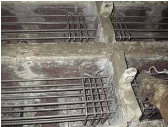
Spiral Wire used in Concrete Railway Sleepers
